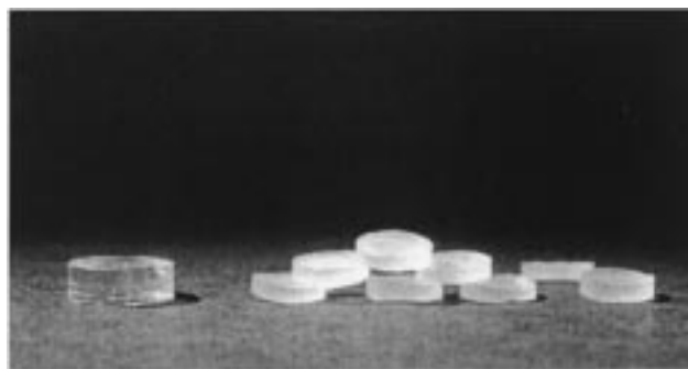
Figure 16. Photograph of 2 mm × 10 mm monolithic polystyrene disks for solid-phase synthesis applications. Shown on the left is a single disk fully swollen in toluene. To the right are a small stack of disks, composition 97% styrene, 3% DVB; note 25 wt % toluene was present in the polymerization to keep the monolith soft enough for cutting.
